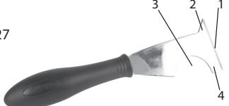
The blade (1) is used to scrape paint and spread compound. The gouge point (2) is used to remove putty/caulk and the curved area (3) is used to clean roller covers. Flat side (4) can also be used to open paint cans.  |                                 |                                                                                                                                                                                  |
