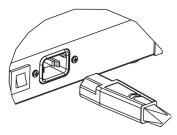
Attach the nut at the end of the air hose to the air outlet on the turbine ensuring it is screwed on fully. The connection will be rigid when fitted correctly.
